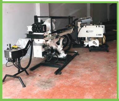
ROTATION UNIT - THE FUNCTIONAL DESIGN OF THE ROTATOR ALLOWS WORKING WITH DIAMETERS FROM B TO N
